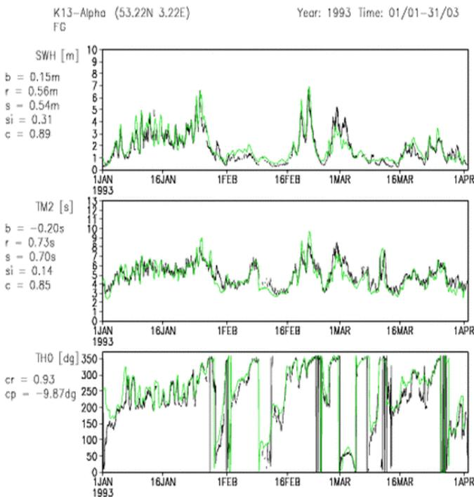
**Figure 4.** Modelled (solid green line) and measured (solid black line) time series for K13-Alpha station in the North Sea (53.2° N, 3.2° E) for the period January to March 93. Model wave data has been produced by the fine grid application of the WAM model for the North Sea. Statistical parameters for the comparison are also shown at the left side of the figure.
